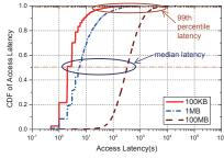
Fig. 2. CDF of access latency when fetching data from the Xuanfeng Cloud CDN.
